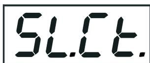
This function allows you to control the slaves from the master's control panel in a master/slave operation. Select this function from the main menu and press [Enter]-button.Browse the list of all connected slaves ("SL.C.1" - "SL.C.9") by pressing [Up] or [Down] button.Select the desired slave and press [Enter]-button.The slave's control panel is available from the master's control panel.
